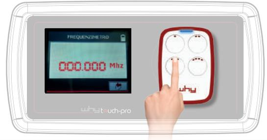
Read on the display the remote control frequency
