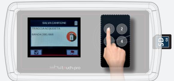
Press the icon at the lower left to save the track on the SD card placed in advance in the designated area.
