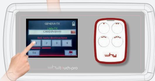
At this moment press at the same time the the 1 and 4 buttons of the Why Evo until when it will start to flash blue and white; so place it on the designated area of the programmer and press OK.
