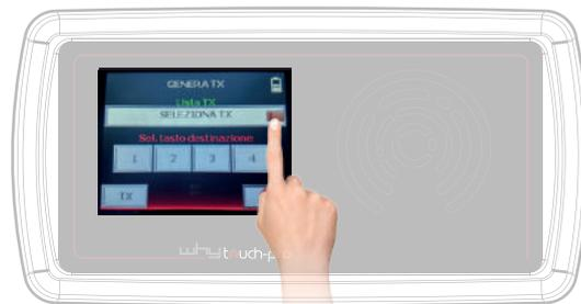
Select through the arrows the model of the desired remote control to be generated
