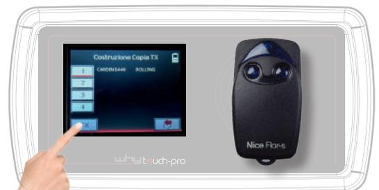
Press at the same time the buttons 1 and 4 of WHY EVO until when it starts to flash blue and white; so place it on the designated area of the programmer and press OK.
