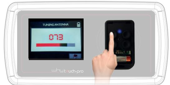
Calibrate with the help of a ceramic screwdriver the "power" of the low frequency remote controls until they reach the highest possible value
